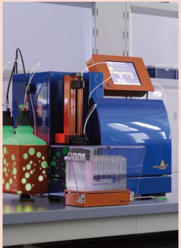
The autoMACS Pro Separator—a compact benchtop instrument
