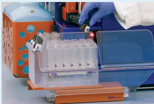
MACS® Reagents are automatically recognized by the barcode reader that allows the software to upload corresponding cell labeling and separation protocols
